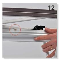
12. We attach the lighting system on structure, inserting it into the 2 clips as in the picture.
